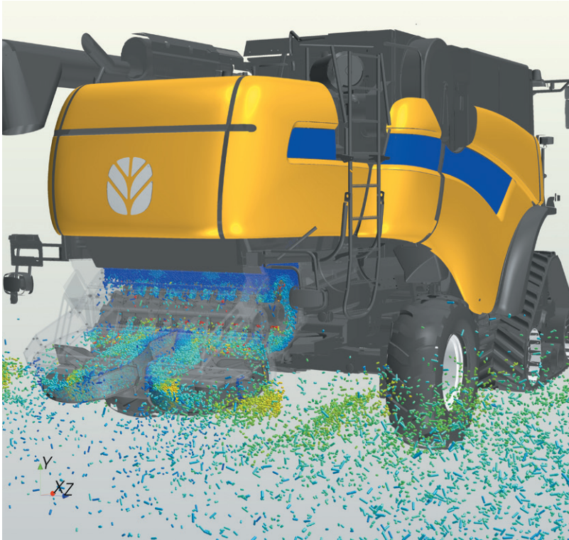
Residue handling simulation on a combine using the discrete element method. (Courtesy of CNH Belgium N.V.)
