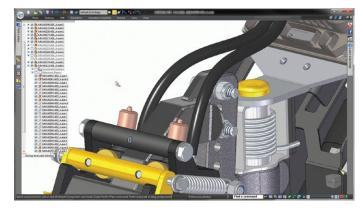
Best-in-class CAD systems like Solid Edge® software also support occurrence property options, which allow you to cull components such as bolts and fasteners from upper-level assembly models.
